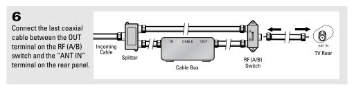
After you've made this connection, set the A/B switch to the "A" position for normal viewing. Set the A/B switch to the "B" position to view scrambled channels. (When you set the A/B switch to "B", you will need to tune your TV to the cable box's output channel, which is usually channel 3 or 4.)
